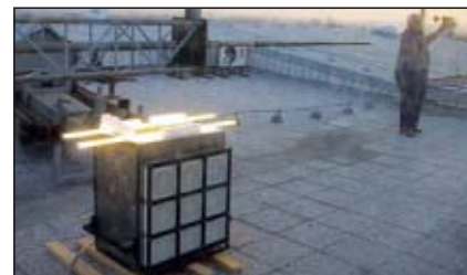
▲ Fig. 8 Upside-down operation, testing for stray radiation.
