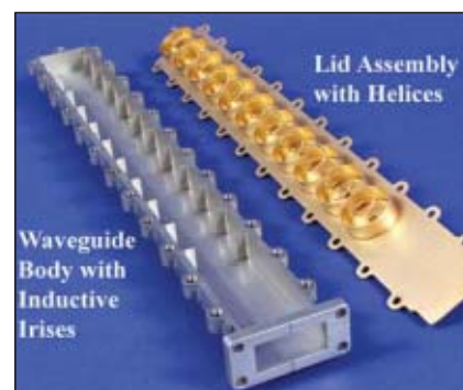
▲ Fig. 5 The lid assembly and waveguide body for the 7.2 GHz array.
