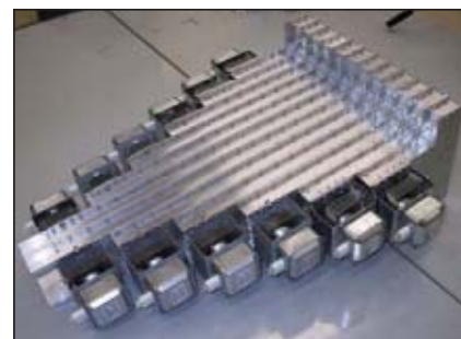
▲ Fig. 4 The installed magnetrons.
