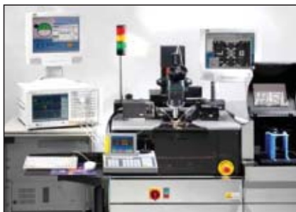
▲ Fig. 1 The automated multiport wafer level measurement system consisting of the probe system, a multiport VNA, calibration substrates, wafer probes, a control PC with software and interfaces between the PC, probe system and VNA.
